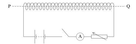
The magnetic flux density B is investigated along the line PQ. Typical results are shown on the graph below. The distance AB represents the region inside the solenoid.
