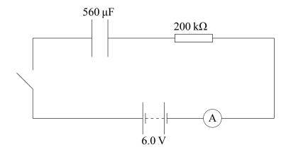
The switch is closed. Some time later the ammeter reads 20  $\mu A$ .
