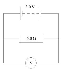
(i) The very high resistance voltmeter gives a reading of 2.8 V. Show that the internal resistance of the battery is about  $0.4 \Omega$ .
