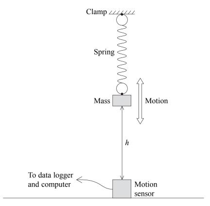
The data logger records how the height h of the mass above the sensor varies with the time t. The computer calculates the velocity v and acceleration a and displays graphs of h, v and a against t. Idealised graphs of h and h for two cycles are shown opposite.
