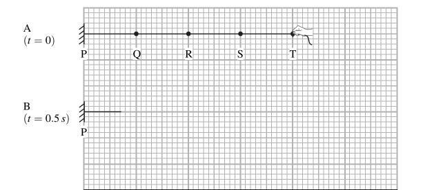
The teacher grasps knot T and pulls it away from P at a steady speed of  $0.80\,\mathrm{m\,s^{-1}}$ . The cord stretches uniformly.
