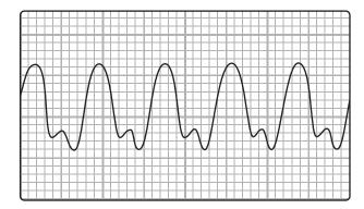
The settings on the oscilloscope are: vertically  $50\,\mathrm{mV\,cm^{-1}}$  horizontally  $2.0\,\mathrm{ms\,cm^{-1}}$
