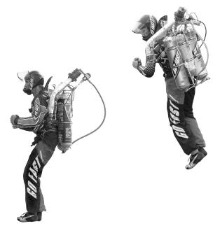
Some jetpacks contain hydrogen peroxide. The hydrogen peroxide decomposes rapidly to form oxygen and water. This rapid release of oxygen from the jetpack lifts the person off the ground.
