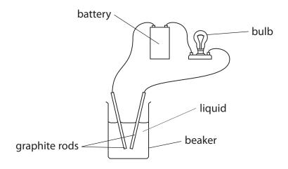
Describe how you would use this apparatus to show that the electrical conductivity of hexane is that of a typical simple molecular, covalent compound.
