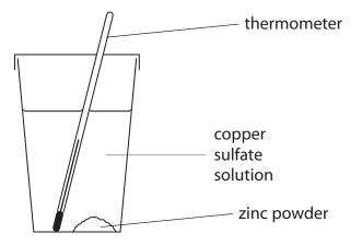
The zinc powder reacts with the copper sulfate solution to produce zinc sulfate solution and copper.
