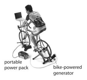
(i) The output voltage of the generator is 12.3 V. The output current is 8.00 A.
