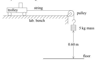
She starts her trolley from rest and uses a data logger to measure the acceleration. Fawzia finds that the acceleration is  $7.92 \text{ m/s}^2$ .
